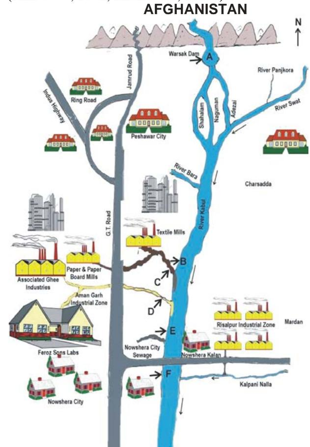
Fig. 2. Water sampling points at Warsak Dam (A) main river (B, E, F) and factories drains (C, D) along River Kabul.
